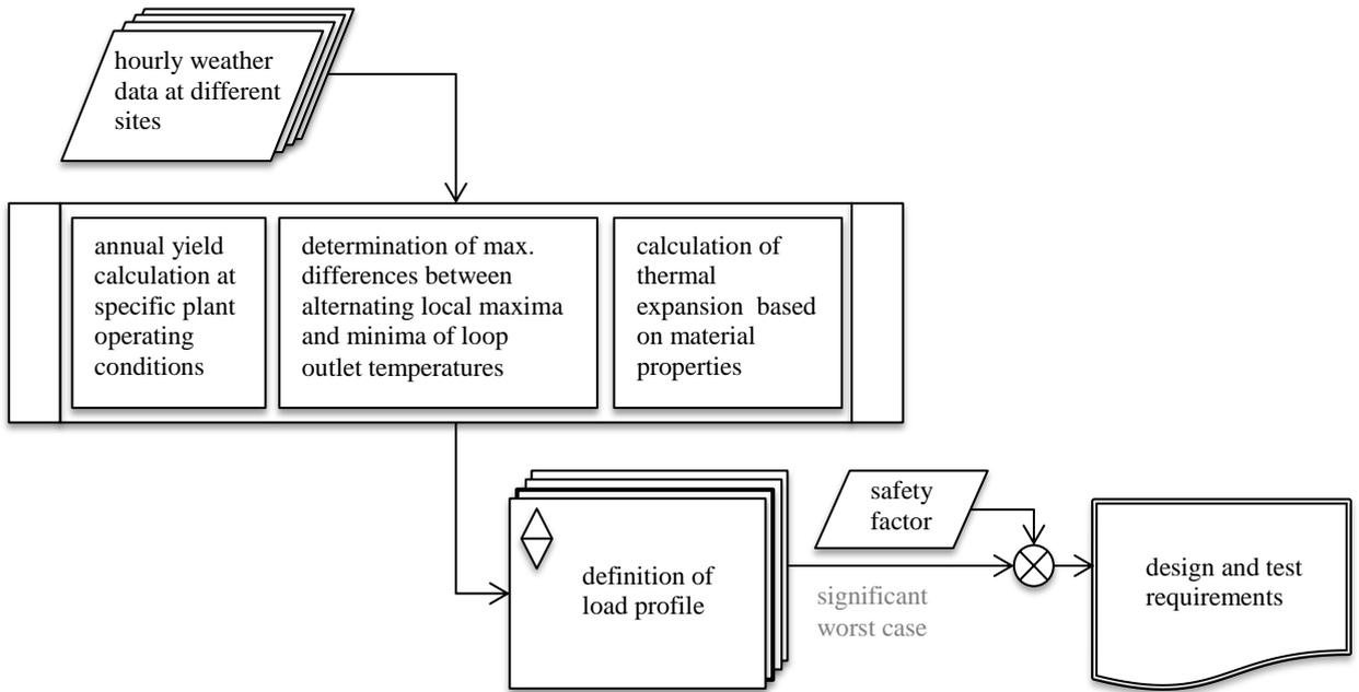
Fig. 2. Process of compensator requirement definition based on specific power plant location and operation conditions
