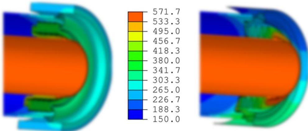
Fig. 3. Temperature distribution on receiver ends at (a) SCHOTT 3<sup>rd</sup> Generation receiver; (b) SCHOTT 4<sup>th</sup> Generation receiver [3].
