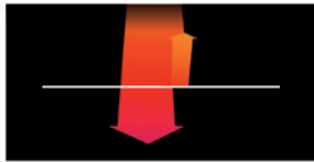
2. ROBAX® Energy Plus reflects more heat radiation than a non-coated ROBAX® panel.
