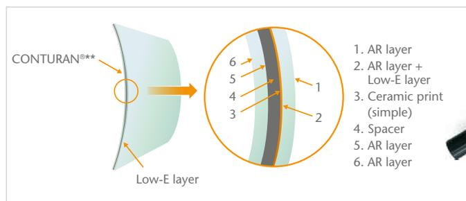
\*\* Sample glass set-up for bent double glazing units. Low-E layer also on level 3 possible.
