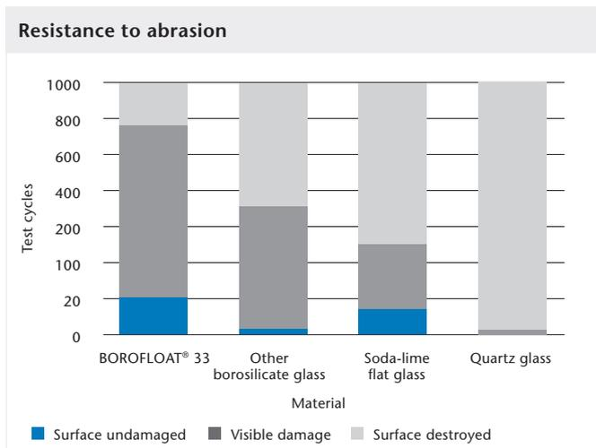
According to a study conducted by the Fraunhofer Institute for Applied Optics and Precision Engineering, BOROFLOAT® 33 displayed the highest resistance to mechanical forces in comparison to other Materials.
