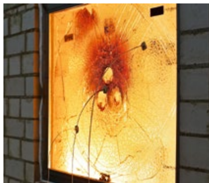
Test: Large fire test after gun shots
