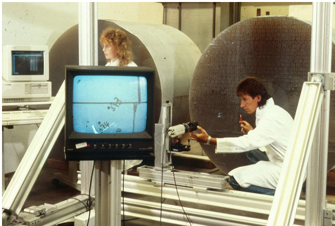
Fig. 7: Focal scanning of large thickness ZERODUR® boules with an IR sensitive CCD camera (for AXAF/Chandra)
