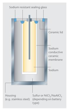
Other sodium-resistant sealing glasses covering the CTE range of 5.5 to 8.5  $10^{-6}$  K<sup>-1</sup> available upon request. Optionally up to 30 Vol.% of an oxidic filler may be added to adapt the properties.
