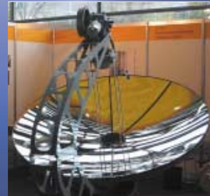
Parabolic mirror for driving Stirling motors
