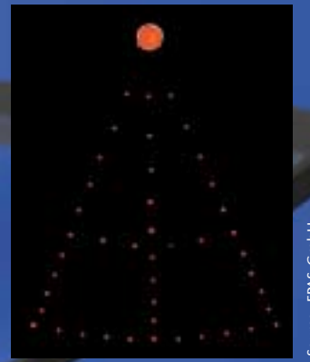
Test chart for a parabolic mirror section ( \phi of the focal point 40 mm)
