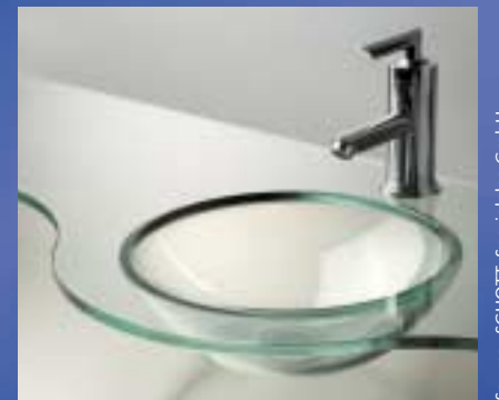
FRANZISCA wash basin made of glass, with the sink mounted underneath the surface area. Both parts thermally toughened.
