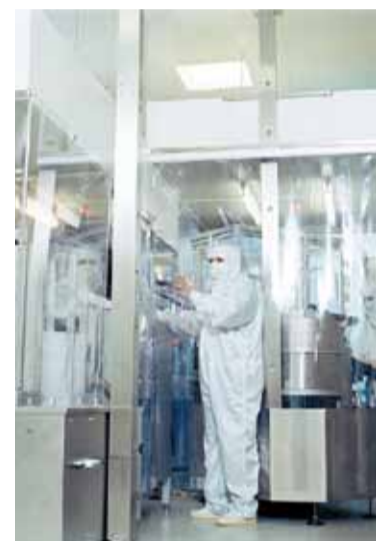
forma 3 + prefillable syringes are produced under clean room conditions.
