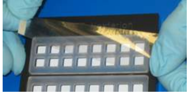
Fig. 4 Seal reaction chambers
