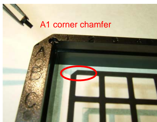
Step 2: Insert patterned plate upright into tray cavity with chamfered corner in the A1 position and secure with the 4 pins, one in each corner.
