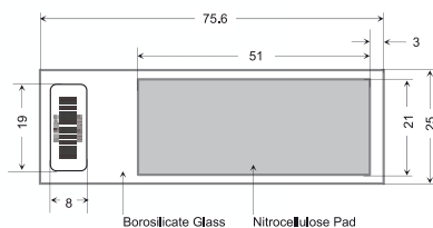
Dimensions of Nexterion® Slide NC single pad
