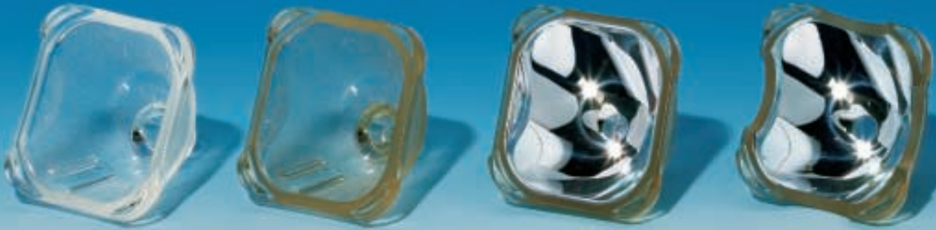
The four production stages of a high-tech reflector (from right to left): pressed green glass, ceramized blank with zero thermal expansion, PICVD-coated dish, finished reflector.
