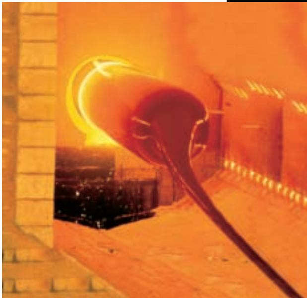
A continuous strand of molten glass flows onto the slowly rotating Danner mandrel. At the lower end the already formed tubular glass is drawn off and directed horizontally.
