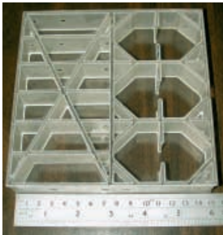
Test structure with "Zerodur" glass-ceramic for mechanical EUVL components.
