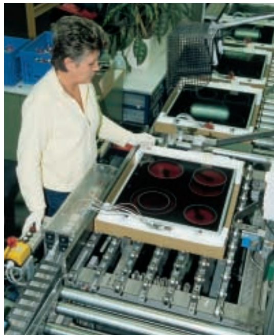
Every glass ceramic cooktop is carefully checked before being set into the appliance.
