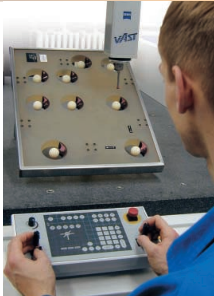
Technicians and calibration laboratories choose this device most often: The 2-D ball disks with bores and extremely precise ceramic balls.
