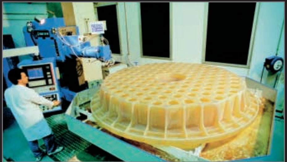
A honeycomb structure has been milled out of the reverse side of the "Zerodur" mirror blank, reducing its weight from four tonnes to 850 kilograms.
