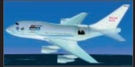
SOFIA airborne telescope: the optical instrument is installed in the Boeing 747's fuselage.
