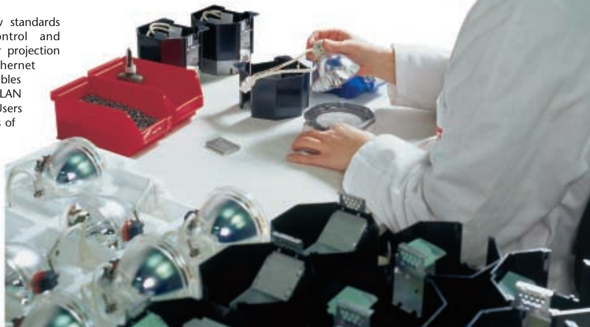
Schott Auer reflectors are inserted in the lamp housing.
