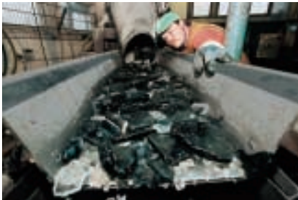
The processing of mixed glass from picture tubes involves separation, cleaning and optical sorting.
