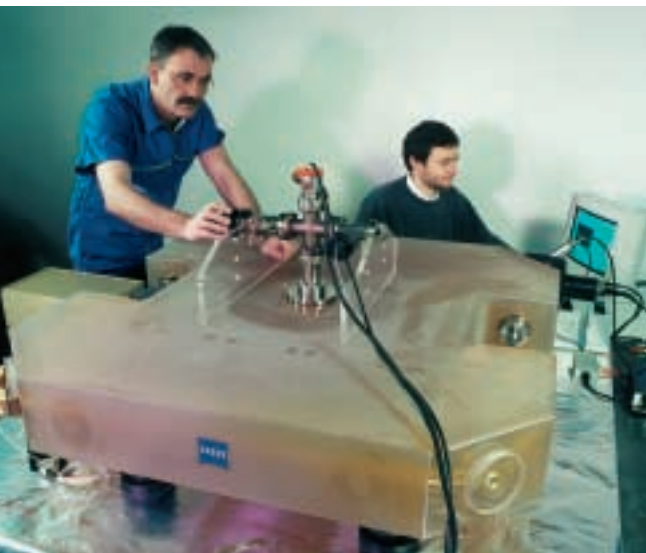
Successful measuring tests have been carried out in New Zealand using a prototype ring laser made at Zeiss and incorporating "Zerodur".
