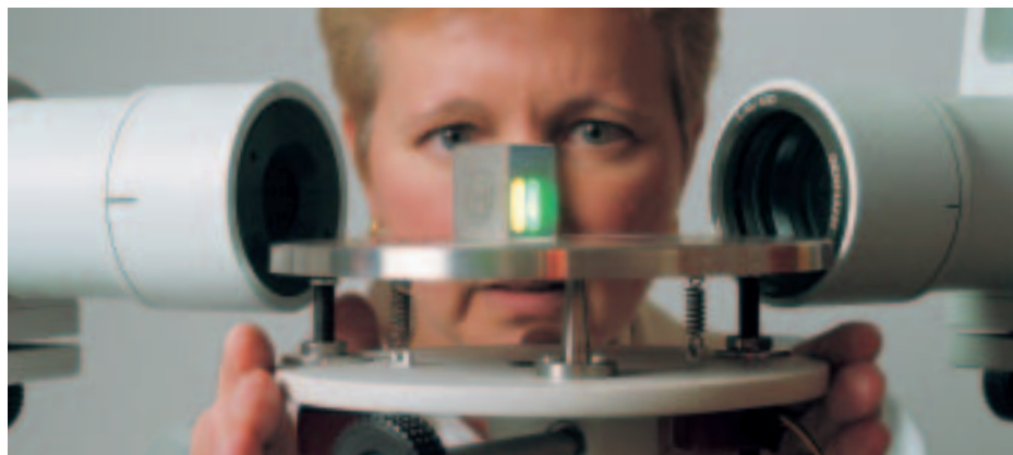
The testing device shown above can determine the exact optical properties of a prisma.
