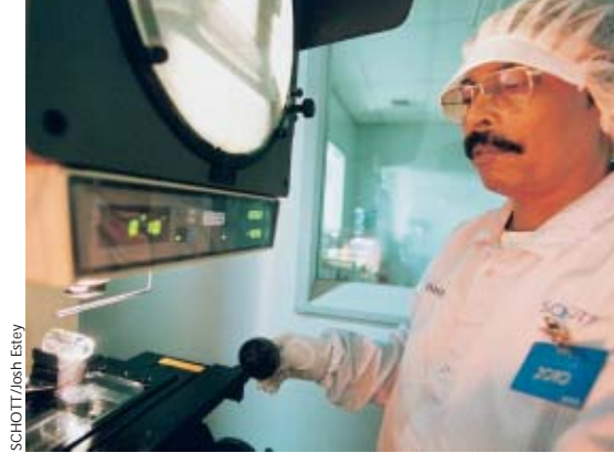
A profile projector measures the geometry of the glass object – optically and without contact.
