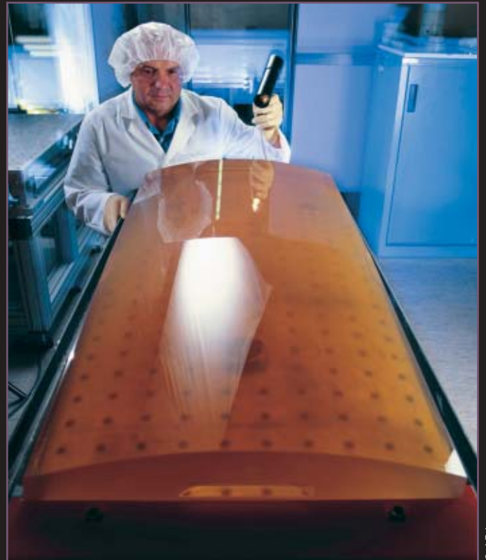
For the "Constellation X" X-ray telescope commissioned by NASA, SCHOTT Glas produced a so-called mandrel for Zeiss, with which the mirror segments can be reproduced.
