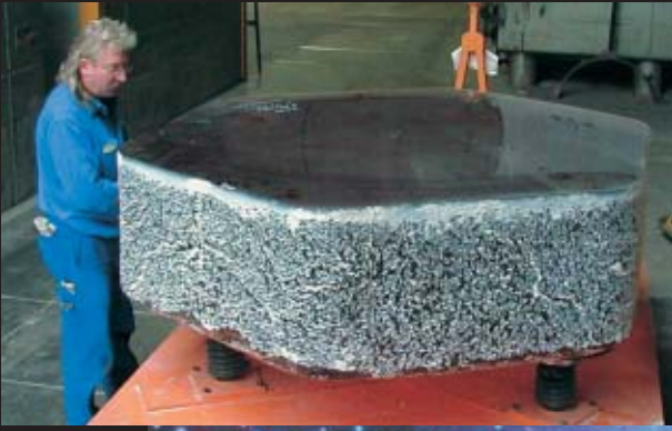
With a process developed by SCHOTT, "Zerodur" blocks can be directly cast as hexagonal blanks.
