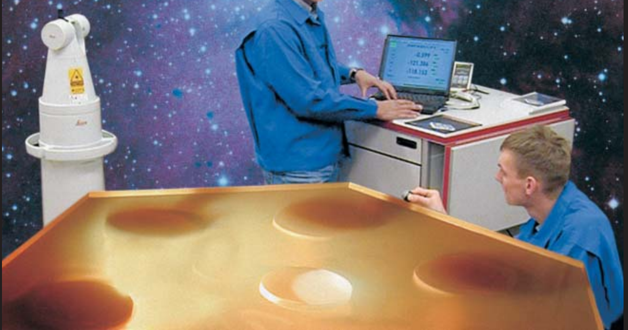
Laser-aided measuring instruments detect the slightest deviations from the control values.
