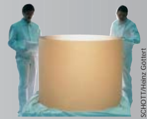
Mirror cylinders made from "Zerodur" glass ceramic for the ROSAT X-ray telescope, and later also the "Chandra" telescope.
