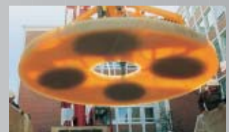
4.1-meter mirror substrate for VISTA, the most powerful wide field survey telescope in the world.
