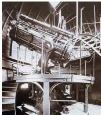
The first mirror telescope of the University of Heidelberg began operations on the Königsstuhl in 1906. The mirror substrate from SCHOTT measured 720 mm.
