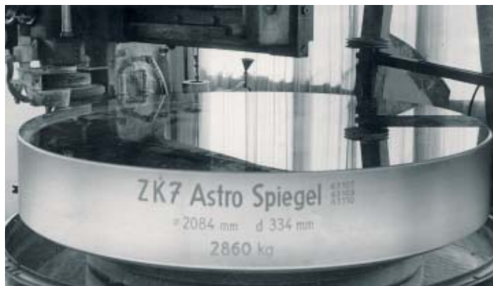
The first postwar mirror substrate that SCHOTT produced from ZK 7 optical glass in 1949 weighed three tons.
