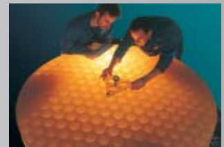
Weight-reduced, "honeycombed" mirror substrates made from "Zerodur" glass ceramic are used in the "Magellan" telescope.
