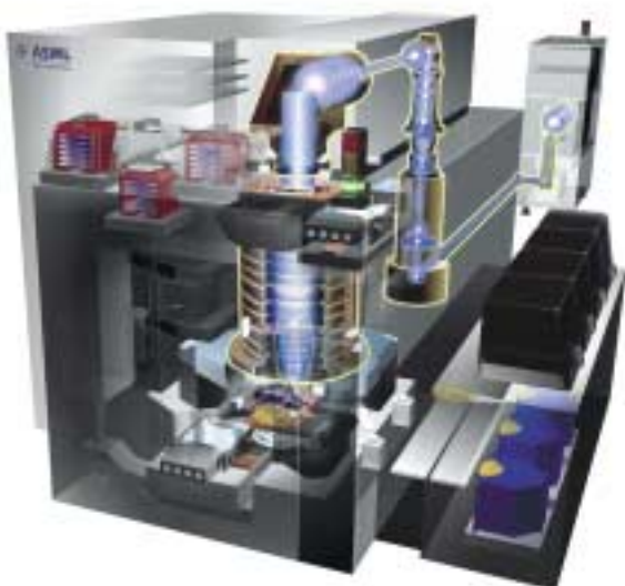
A schematic drawing of an ASML wafer stepper (left). The U.S. company Cymer has recently developed even more efficient excimer lasers with its innovative XLA 100 system and so-called “MOPA technology.”
