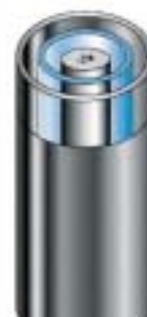
A primary component of ozone generators are the glass tubes, each of which contains a metal rod. The glass tubes are enclosed by stainless steel sheaths. Ozone is produced from pure oxygen by applying electric voltage to the chambers between the metal rod and the metal sheathing.
