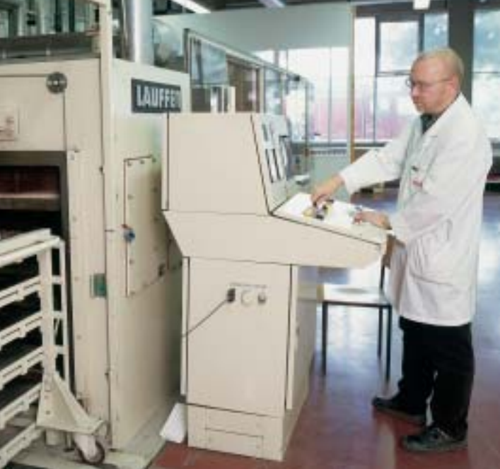
The laminate preforms are processed in the press at temperatures of 180° C to 200° C.
