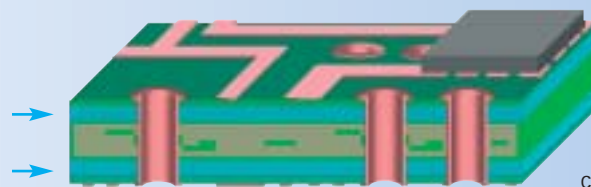
The structure of a multilayer laminate: a copper foil is clad to both sides of the thin glass with the help of a resin. Intermediate layers made from glass fiber-reinforced adhesive join the other layers.
