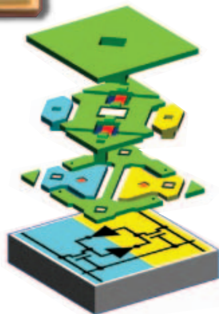
The mini-reflectors on the DMD chip can change their position in less than one millionth of a second.
