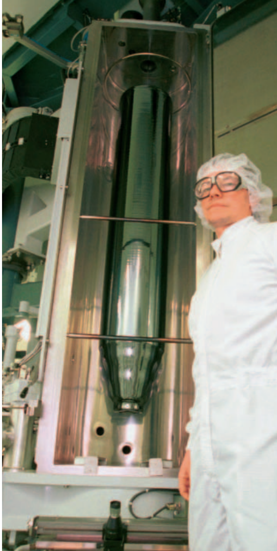
State-of-the-art: Crystal growth facility for the manufacture of 300-millimeter diameter silicon monocrystals at Wacker Siltronic AG.
