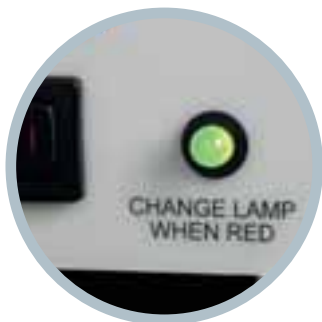
Lamp change indicator shows when halogen bulb needs replacement
