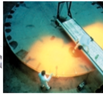
The biggest glass item in the world cast in one piece: diameter 8.2 meters
