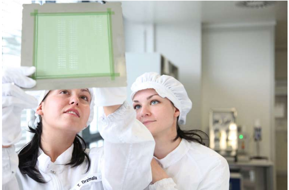
Quality control of the preliminary products ("greensheets") for manufacturing multilayer ceramics.
