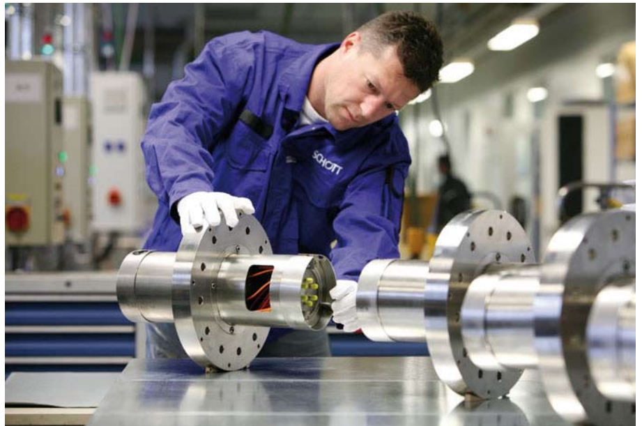
Attenuation measurement of fiber optical penetrations for pressurized water reactors (PWR) and boiling water reactors (BWR).
