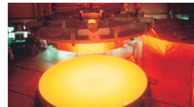
A crowning achievement: an eight-meter mirror carrier. Four of these "Zerodur" mirror carrier form the core component of the world's most powerful telescope, the Very Large Telescope (VLT) in Chile.
