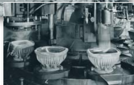
Since 1955 fully automated: Television glass manufacture in the main works in Mainz.
