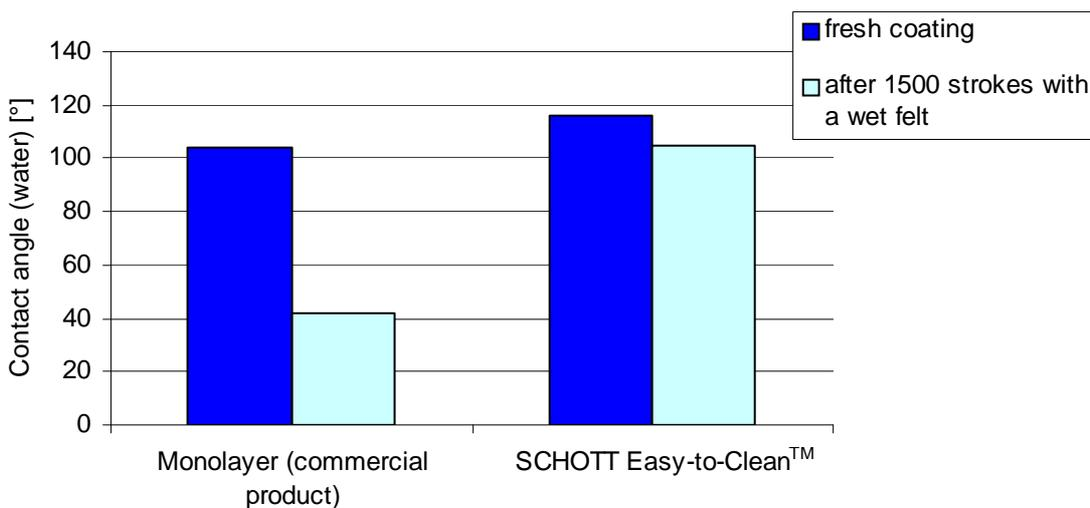
Figure 4: Progression of the contact angle following the stress of the scrubbing test
