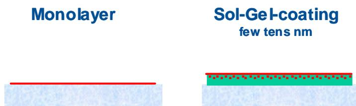
Figure 2: Approaches for easy-to-clean coatings
