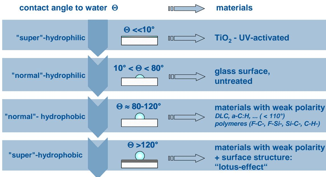
Figure 1: Wetting behaviour of easy-to-clean surfaces
