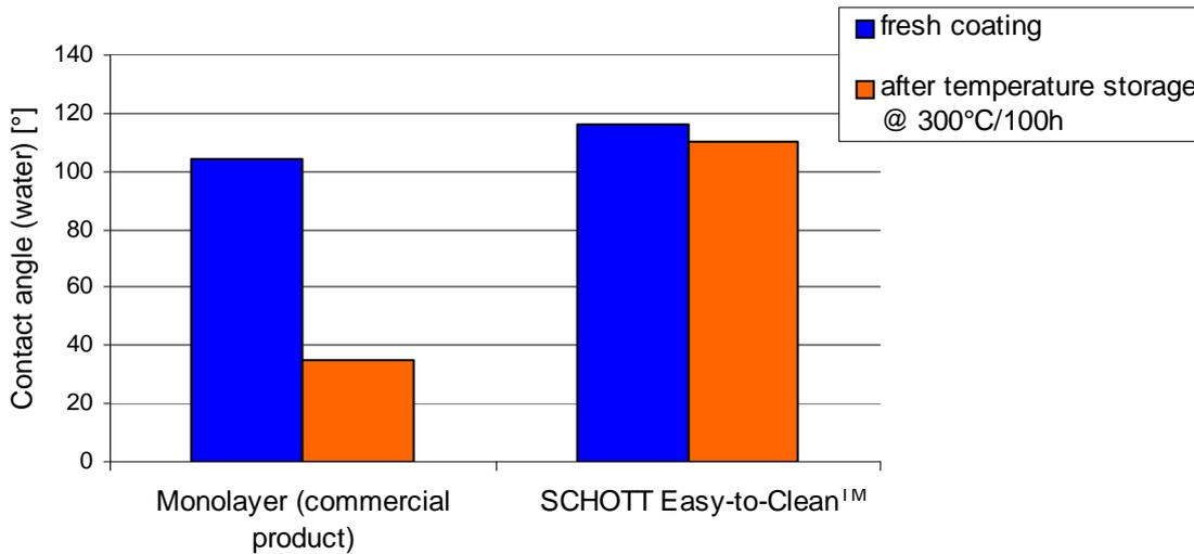
Figure 3: Comparison of surface properties under thermal stress
