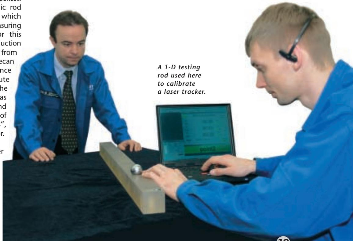
*A 1-D testing rod used here to calibrate a laser tracker.*
