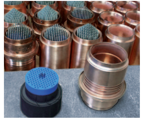
Assembly of Control and Instrumentation (C&I) penetrations for nuclear power plants prior to sealing.
