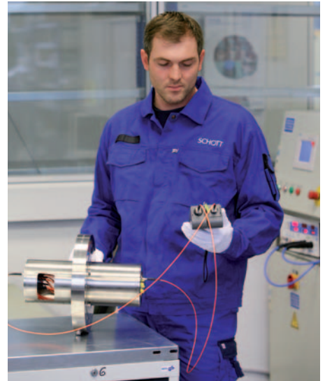
Measurement of glass-to-metal sealed penetrations for PWR and BWR
