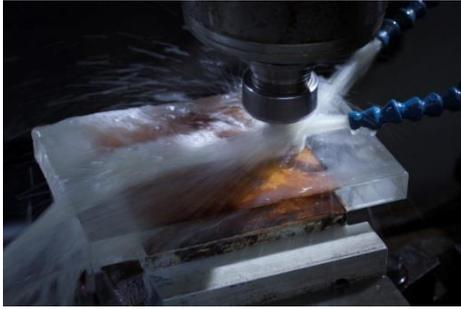
Post-processing of SCHOTT's BOROFLOAT® floated borosilicate glass to achieve the smooth surface needed to create optical mirrors. Photo: SCHOTT.
