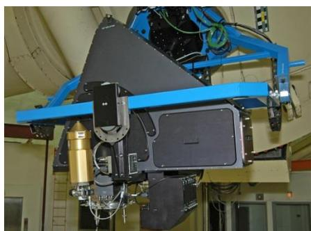
Prototype of the spectrograph used for HEDTEX: It uses optical mirrors based on BOROFLOAT® glass from SCHOTT. Source: Courtesy of Martin Harris/McDonald.
