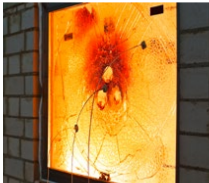
Test: Large fire test after gun shots
