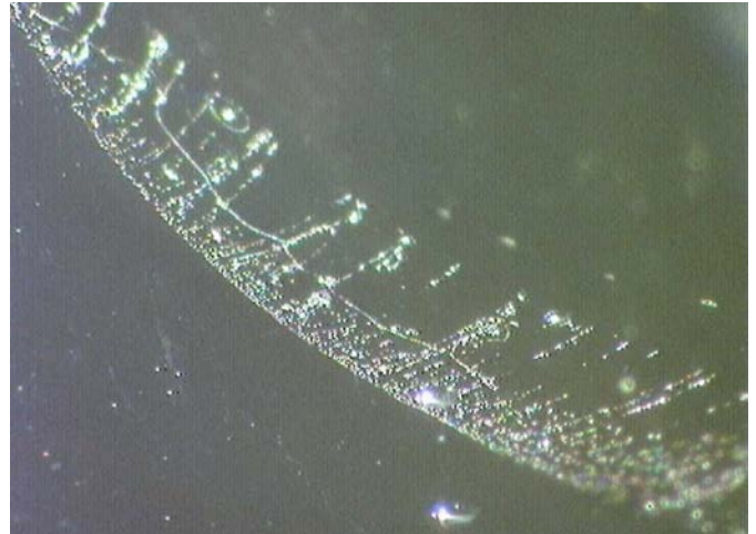
Fig. 2: Bubbles generated by reheat pressing of SCHOTT N-BK7®.
