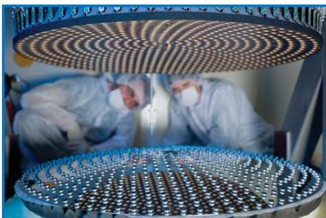
A picture of the movable secondary ZERODUR® mirror during its installation in the Arcetri lab. The image shows the 672 tiny magnets spread over the back of the mirror. The reflecting face of the mirror is face down. The upper portion contains the electro-mechanical devices that control the magnets. Also the support plate serving as precise reference surface for the thin shell is made from ZERODUR®.
