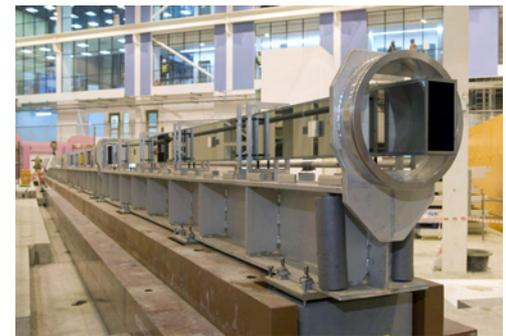
Neutron guides made of double elliptic bended super mirrors
