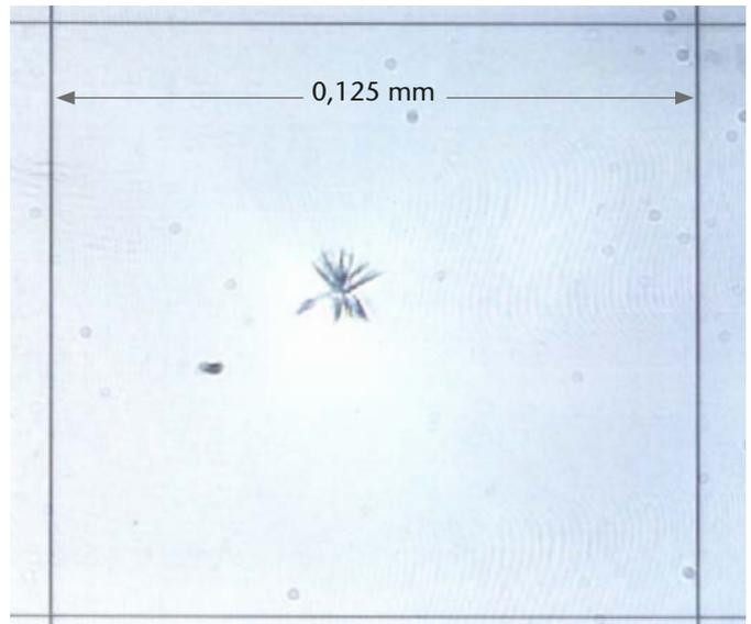
Fig. 3: N-SF6 with crystal due to devitrification
