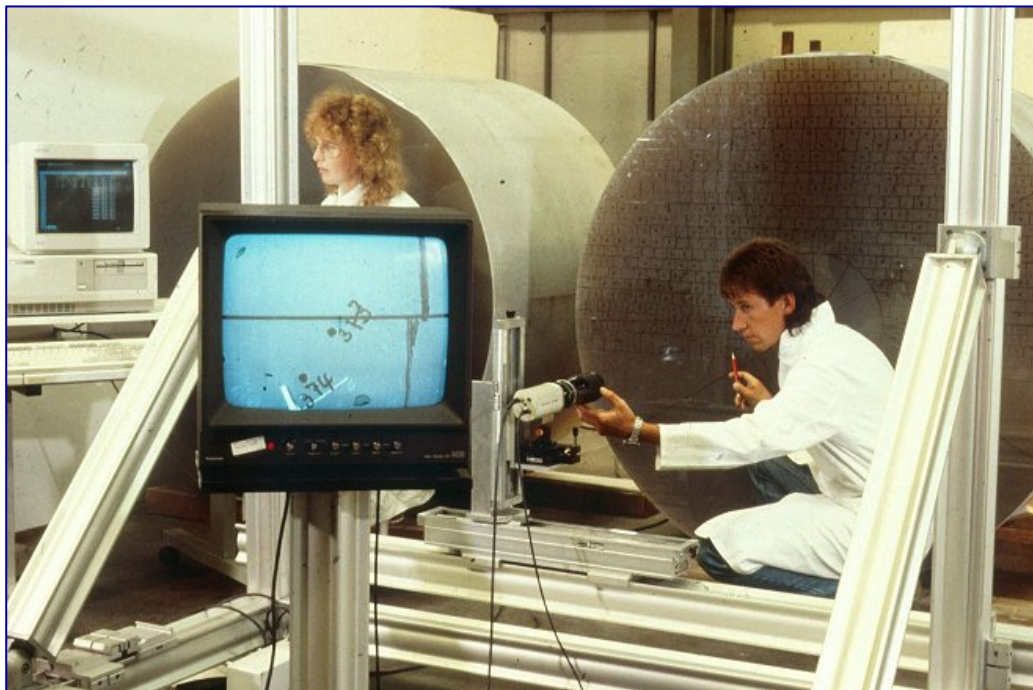
Figure 7: Focal scanning of large thickness ZERODUR® boules with an IR sensitive CCD camera (for AXAF/ Chandra).
