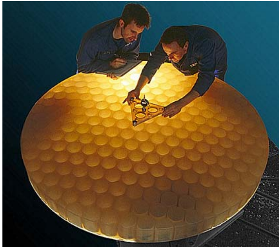
Figure 1: left side: Magellan M2 mirror blank, right side: SEVIRI Scan mirror
