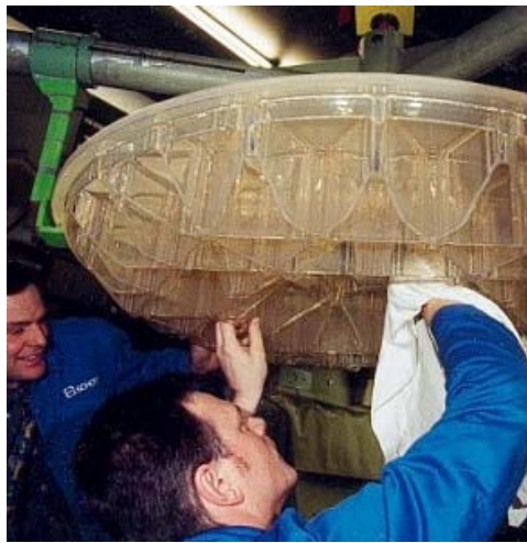
Figure 9: The Gemini M2 mirror blank acid etched to a final weight reduction of 85%.
