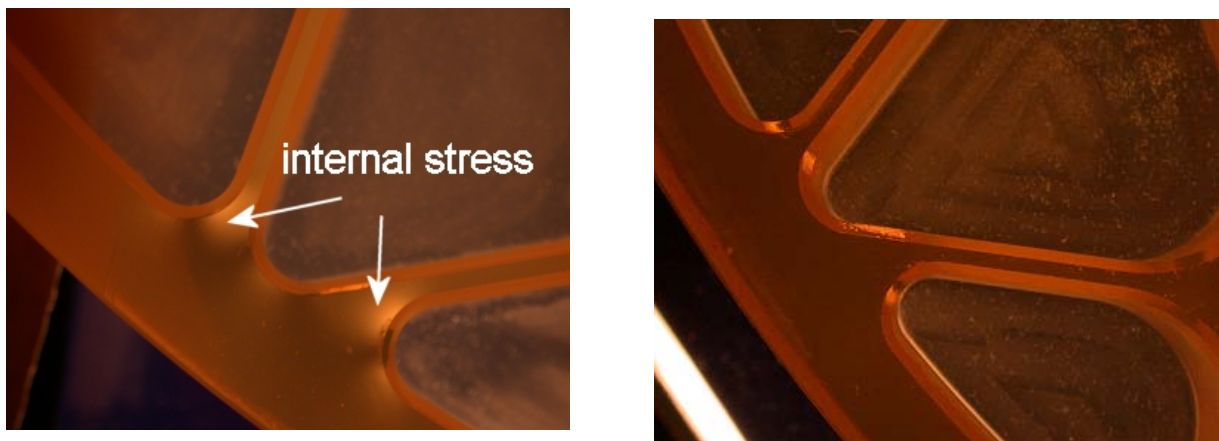
Figure 8: left: lightweight structure with internal stress visible between crossed polarizers. Right: the same structure as seen between crossed polarizers after acid etching.
