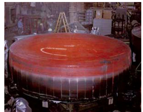
One of the earliest 4 meter ZERODUR® meltings in the beginning of the 70's. Since then equipment and processes have been modified significantly to meet the market's requirements.
