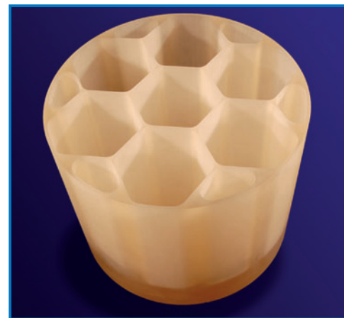
Rib thickness of 2 mm and pocket depths of 190 mm achieved on a 300 mm diameter demonstrator with standard diamond tool grinding
